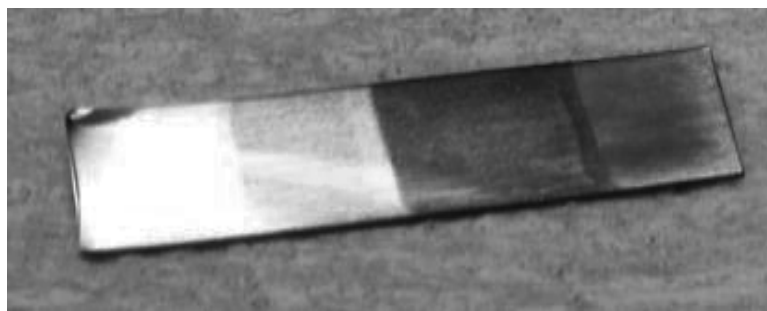
Fig.2 Ag plate of (a) the non-dipped, (b) 5 sec, (c) 10 sec and (d) 15 sec dipped in the mixture of potassium sulfide and calcium sulfide.
